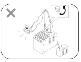
★During use of product, safety valve should not be contacted or opened.
