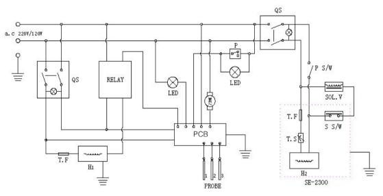
QS: power switch PCB: Pcb board
